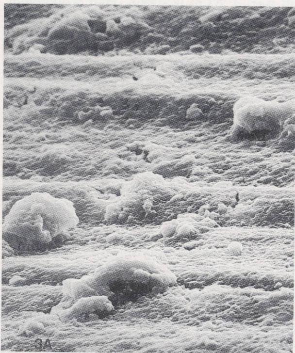
Fig. 3A. A smear layer created using a diamond disc with water coolant. Particle sizes range from 3 to 5 micron. X 6,000.
