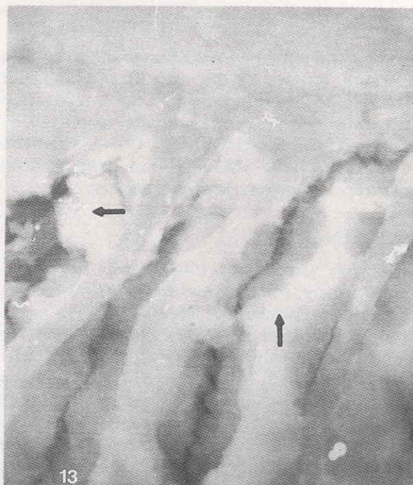
Figs. 12 and 13. Secondary versus Backscattered electron images of an All-Bond 2 specimen stained with silver methenamine. Note the staining around the tags which indicates that collagen is present in that area (arrows). X 3,600.
