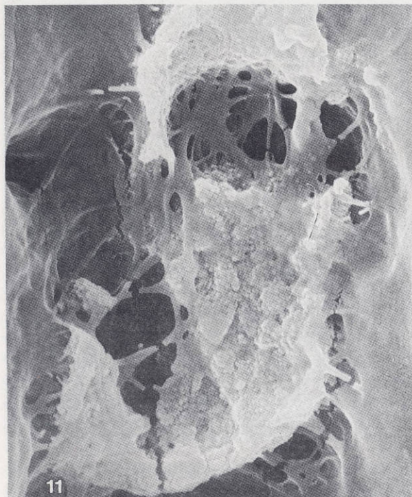
Fig. 11. The same specimen as in Fig. 10 but with the primer applied immediately after treatment with the etching agent. X 18,000.
