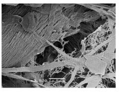
Fig. 3. SEM image of deteriorated cellulose fibers by Scopulariopsis sp.
