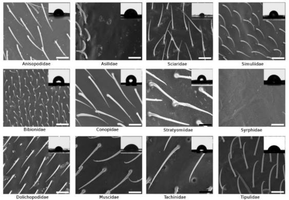
**Fig. 2.** Micrographs of Dipteran wings under SEM with corresponding pictures (inserted) of a water droplet on dorsal surface. Electrochemistry and Chemical Energy Research Center (CELEQ), University of Costa Rica, scale bar: 10um.
