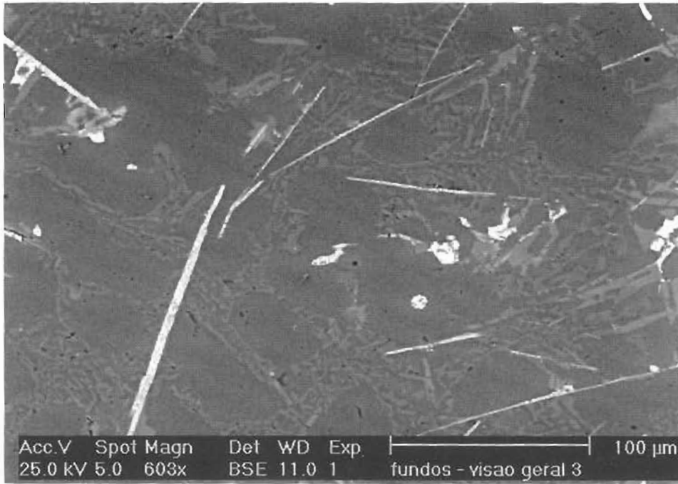
Figure 4- Microstructure image of the experimental alloy obtained by SEM in the BSE mode giving evidence to the differences in the composition of the phases
