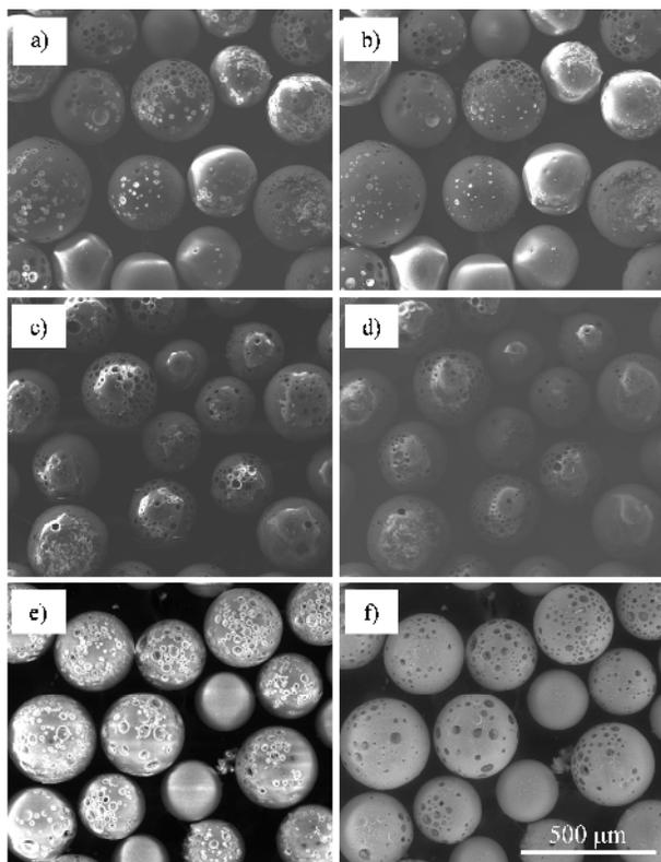
**Fig. 3.** SEM images of a glass sphere acquired as a function of primary electron beam energy: HighVac on uncoated sample a) 30 kV and b) 10kV; HighVac on coated sample c) 30kV and d) 10 kV; and LowVac e) 30 kV and f) 10 kV. Contrast, brightness and focusing of each image were kept constant.
