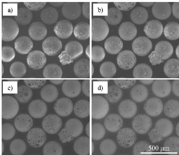
**Fig. 5.** LowVac images of glass-ceramic spheres acquired as a function of gas pressure, P: a) P = 15 Pa, b) P = 20 Pa, c) 50 Pa and d) 80 Pa. The brightness was optimized while other parameters than P were kept constant during image acquisition.
