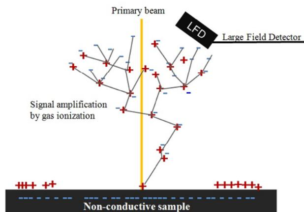
**Fig. 2.** Scheme of charge neutralization process and signal amplification by gas ionization effect.
