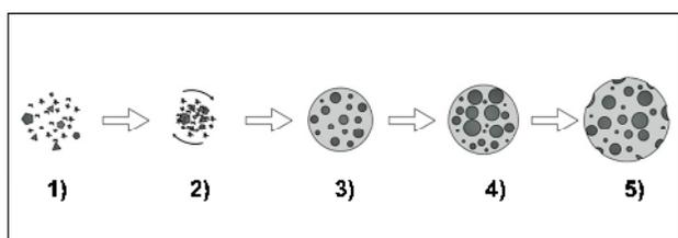
**Fig 1.** Scheme of blast furnace slags (BFS) transformation into glass-ceramic material.
