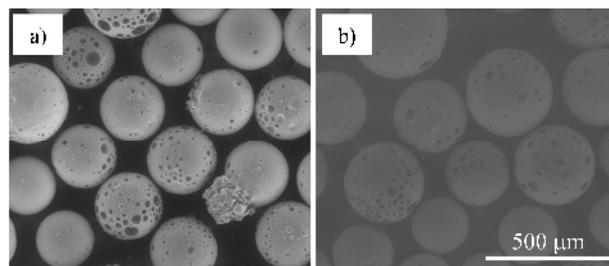
**Fig. 4.** Glass-ceramic spheres images were obtained at different working distance: a) 7.5mm and b) 20mm. The brightness of each image was optimized.
