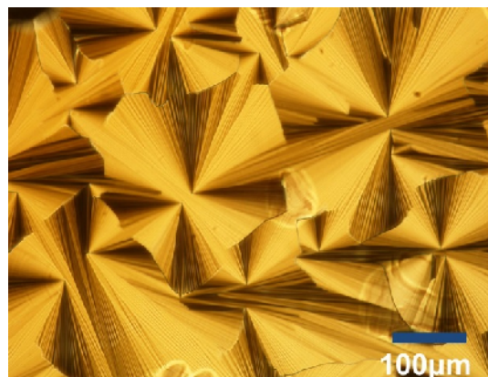
Fig. 2. Polarized light optical microscopy image of the microemulsion sample composed of cylindrical aggregates. The texture is typical of a hexagonal phase.
