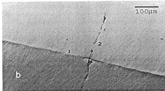
Fig. 6: Optical micrograph of the nitrided steel with a) 75 %; and b) 94 % of fatigue life. (1) surface micro-crack; (2) defect on the nitrided layer. Original magnification: a) 595 X; b) 151 X.
