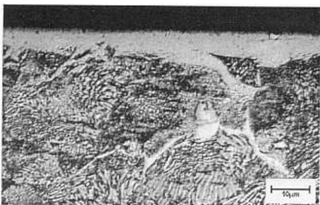
Figure 4 : Photomicrography of alloy 1- Nitrided layer on the as-cast and nitrided substratum constituted by ferrite, and graphite nodules
