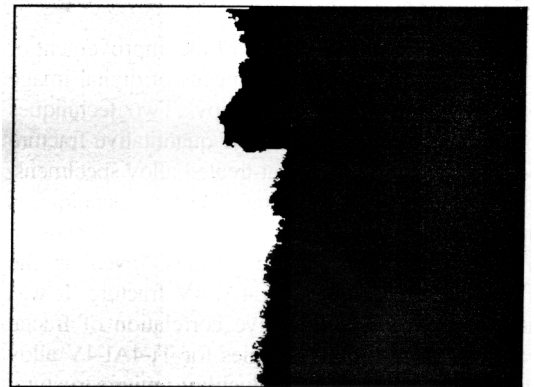
Figure 2. Fracture profile in Figure 1 after Fill Hole filter
