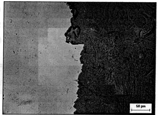
Figure 1. Profile polished of the fractured surface near to Charpy V-notch region.
