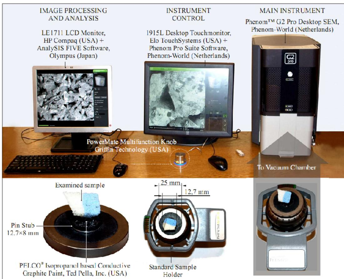
**Fig. 1.** Advanced desktop SEM Phenom G2 Pro produced by Phenom-World: a) general view of the microscopic system, b) general view and details of standard sample holder for non-conductive preparations with a fixed sample prepared for measurements
