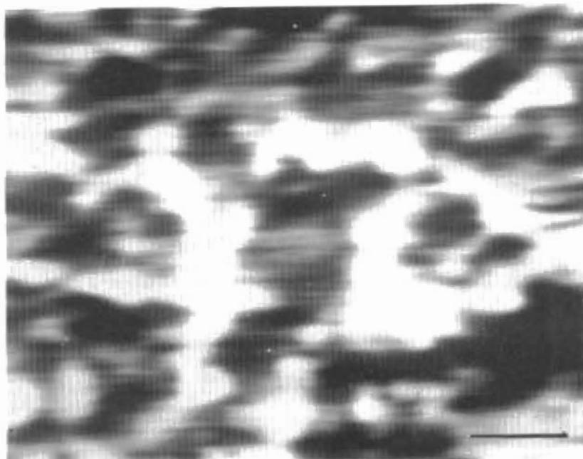
**Figure 5.** SEAM image of sintered  $\text{Bi}_2\text{Sr}_2\text{CaCu}_2\text{O}_x$ . Bar = 50  $\mu\text{m}$ .
