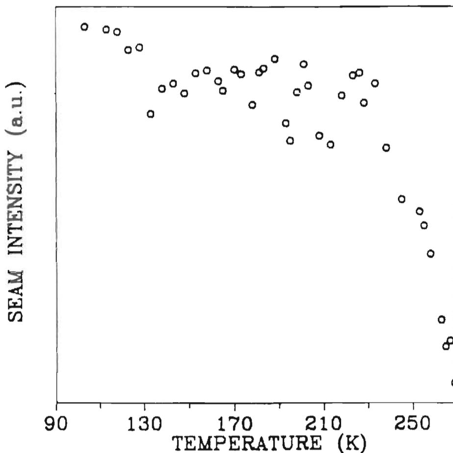
**Figure 6.** Temperature dependence of SEAM signal intensity for a  $\text{YBa}_2\text{Cu}_3\text{O}_{7-x}$  sample.
