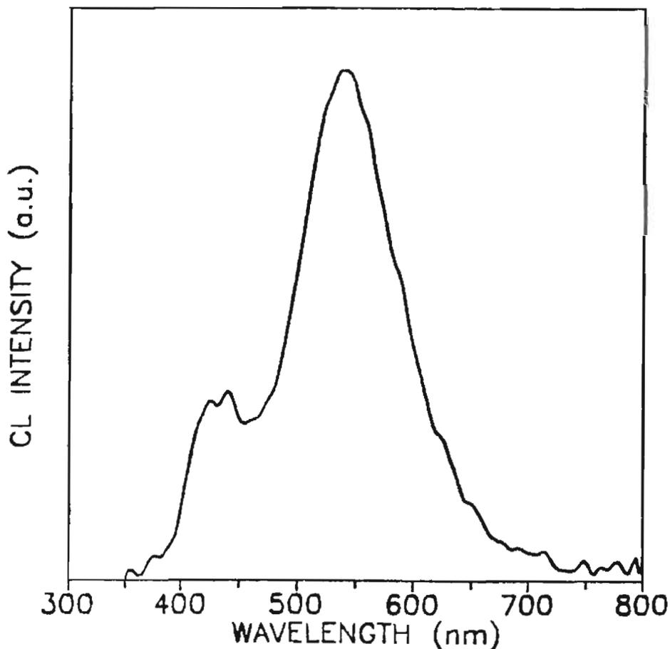
Figure 2. CL spectrum at 110K of an irradiated  $\text{YBa}_2\text{Cu}_3\text{O}_{7-x}$  sample.
