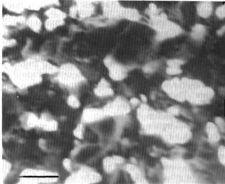
**Figure 3.** CL image of a sintered  $\text{Bi}_2\text{Sr}_2\text{CaCu}_2\text{O}_x$  sample. Bar = 50  $\mu\text{m}$ .
