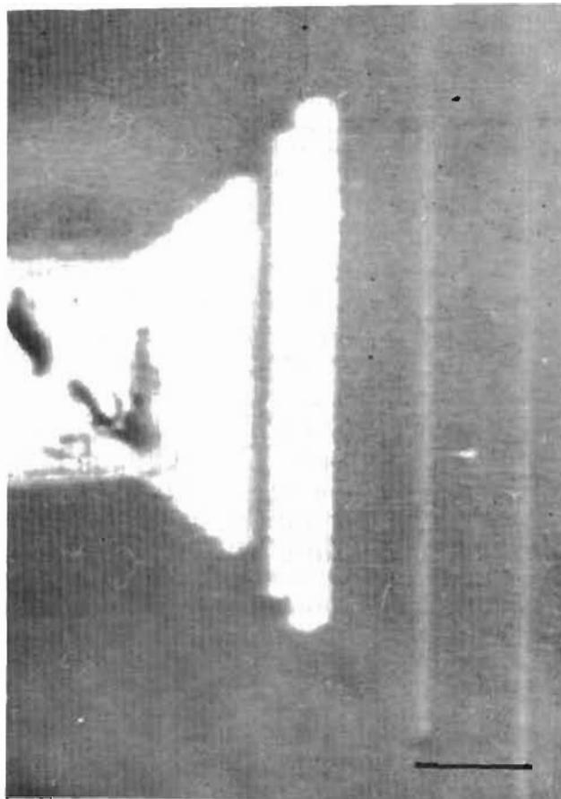
**Figure 1.** Images showing the changes induced by the electron beam on a  $\text{YBa}_2\text{Cu}_3\text{O}_{7-x}$  film (a) emissive mode (b) CL mode. Bar = 50  $\mu\text{m}$ .
