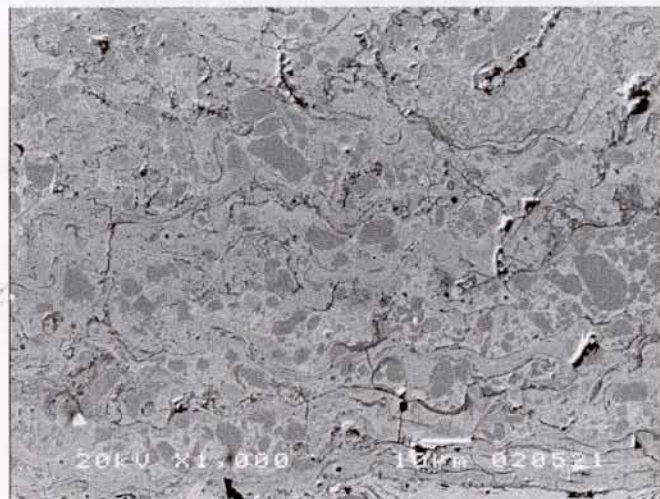
Fig. 2: SEM cross-section image of the thermal treated Q3 sample, close to the substrate.
