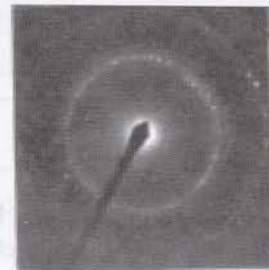
Figure 3 - Electron diffraction pattern triple junction of the grain matrix (point 2) at figure 2.
