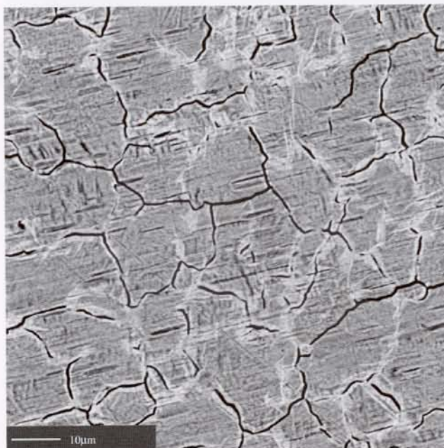
Fig. 3: Backscattered electrons image of the nickel foil just after the hydrogenation.
