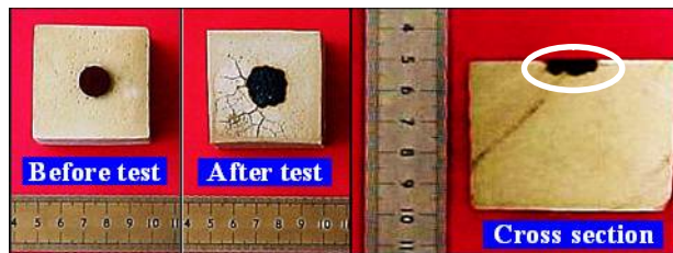
Fig. 3. (A) Reactive pellet / refractory concrete set before the test, (B) Refractory concrete after test and (C) Cross section cut of the set.
