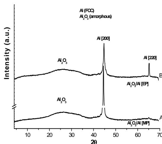
Fig. 2. XRD patterns of the catalytic supports: (A)  $\text{Al}_2\text{O}_3/\text{Al}$  [MP]; (B)  $\text{Al}_2\text{O}_3/\text{Al}$  [EP].
