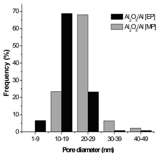
Fig. 3. Pore size distributions of the  $Al_2O_3/Al$  [MP] and  $Al_2O_3/Al$  [EP] supports.
