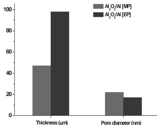
Fig. 1. Relationship between the pretreatments on the aluminum surface and the physical properties on the  $\text{Al}_2\text{O}_3/\text{Al}$  supports.
