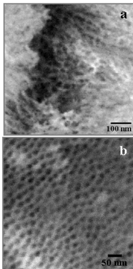
Fig. 4. SEM micrographs of the pore distributions in (a)  $Al_2O_3/Al$  [MP]; (b)  $Al_2O_3/Al$  [EP].
