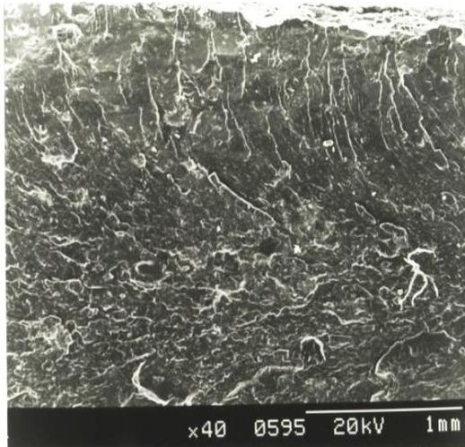
Fig. 5. SEM micrographs taken from the impact fracture surface of PP/SBS 70/30 SV blends.
