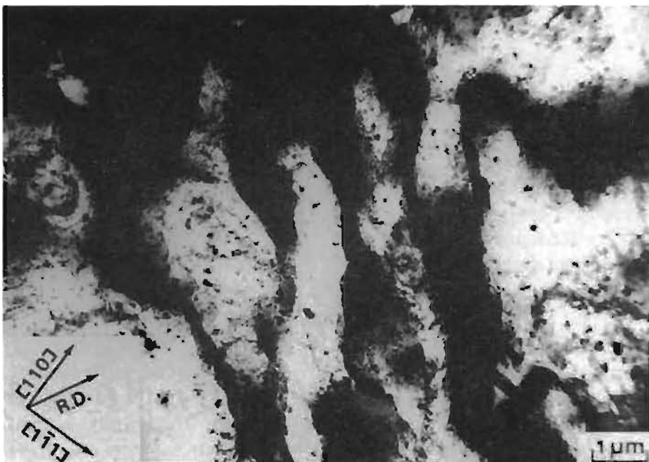
Fig. 16 TEM observation in low carbon steel showing dislocation cells in a specimen predeformed in rolling (0.10) and after being recovered at 600 °C in vacuo for 1 h. The grain has a \langle 112 \rangle axis normal to the sheet plane. (R.D., rolling direction).
