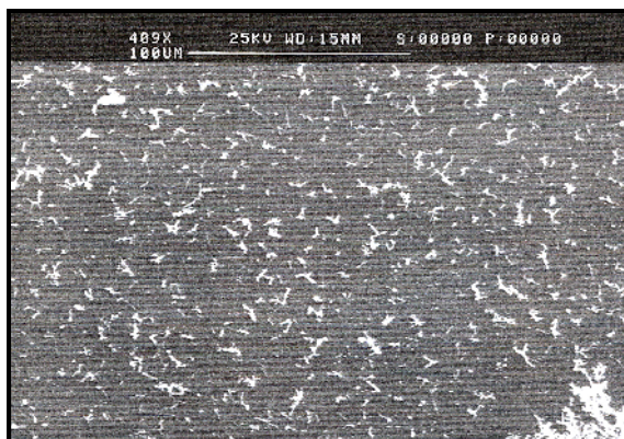
Fig. 8. SEM image of aerosol fibers of caffeine generated with the MAGE for optical measurement purposes. The bar represents 100 \mu\text{m} .
