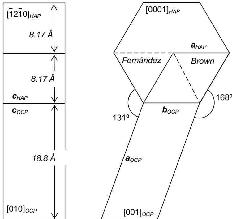
**Fig. 2.** Structural considerations according to the models proposed by Brown [11] and Fernández [12].
