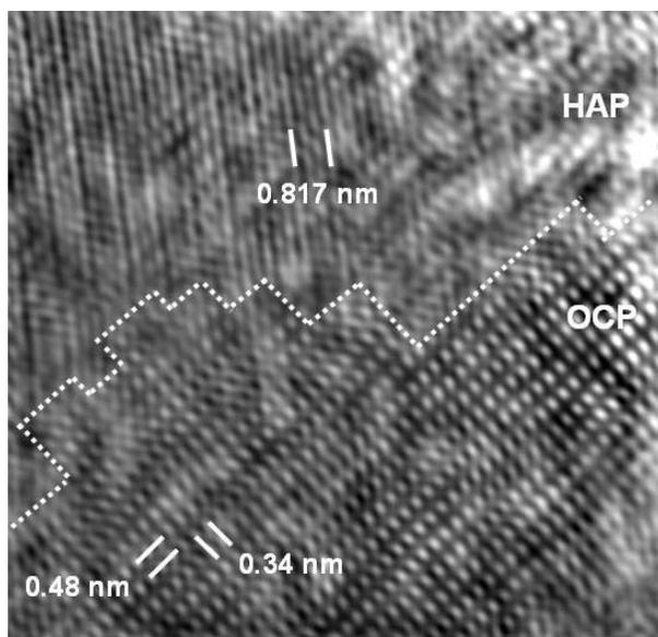
**Fig. 4.** The HRTEM image of a grain of the sample obtained after thirty minutes of hydrolysis where coexistence of HAP and OCP is observed. Dashed lines indicate a boundary between HAP (along the  $[10-10]$  zone axis) and OCP (along the  $[010]$  zone axis) phases.
