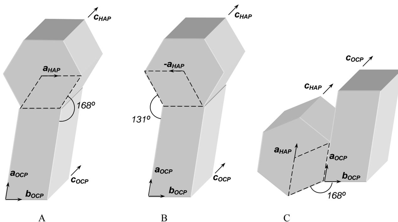
**Fig. 1.** Schematic 3-D presentation of the three models so far available for the OCP-HAP interface. A) Brown [11], B) Fernández [12] and C) Xin [8].
