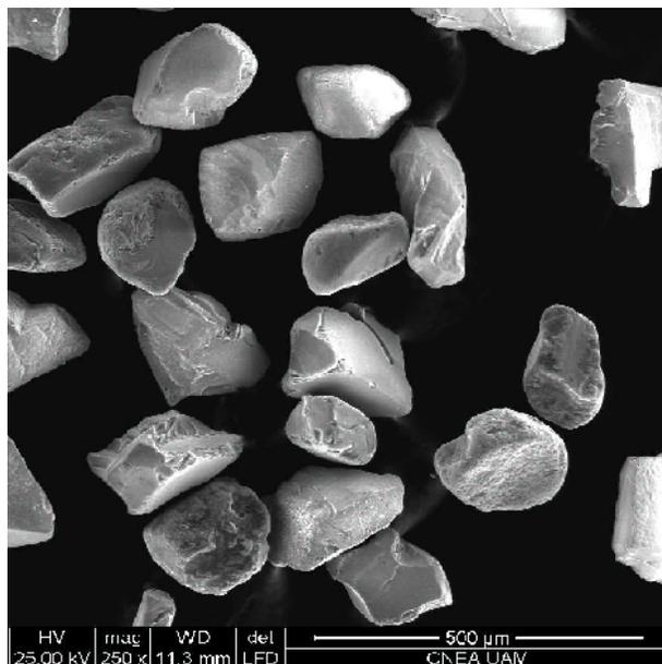
**Fig. 1.** Electron micrograph of rhodesite abrasive particles, obtained with secondary electrons and large field detector.
