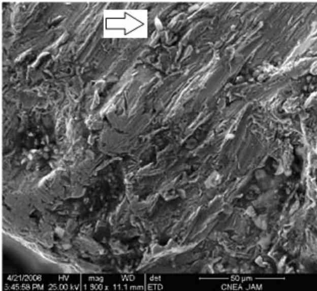
**Fig. 2.** Electron micrograph, of an AISI 304 stainless steel surface cut by WJM, arrow indicates abrasive particle. Using Everhart Thornly detector.
