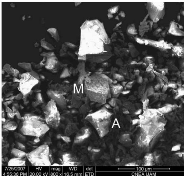
**Fig. 3** Electron micrograph of abrasive (A) and metal (M) particles, obtained with Everhart Thornly detector.
