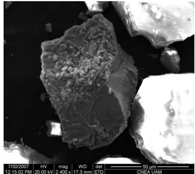
**Fig. 4.** Electron micrograph of metal particles obtained with Everhart Thornly detector.
