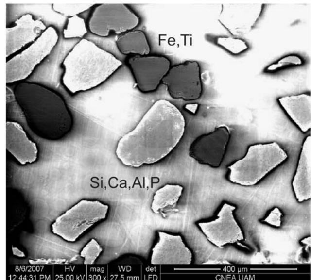
**Fig. 5.** BSE micrograph, showing abrasive (Si, Ca, Al and P) and metal (Fe, Ti) particles, light and dark respectively, obtained with large field detector.
