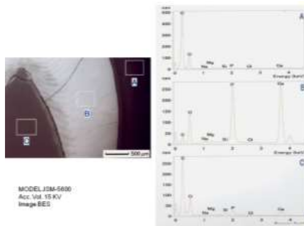
Fig. 7. SEM image in backscattered electron mode of the adult human tooth sample after thinning it to a thickness of 100 \mu\text{m} , approximately, mirror polishing and chemical etching. A-C) EDS spectra of the areas indicated by the boxes in the SEM image. A) Resin area where the tooth was immersed for its thinning and mirror polishing process. B) Enamel, C) Dentin.
