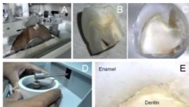
Fig. 3. Illustration of the human tooth sample preparation procedure. A) Cutting with a diamond disc. B) Human tooth after cutting. C) Immersion of the tooth into a resin to carry out the mechanical grinding. D) Thinning and polishing by mechanical grinding with SiC sandpaper. E) Human tooth sample after mirror polishing and chemical etching.
