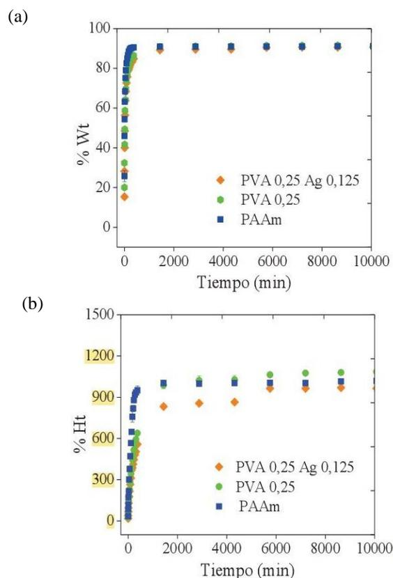
**Fig. 2.** Swelling isotherms as a function of time: a) adsorbed water b) swelling index
