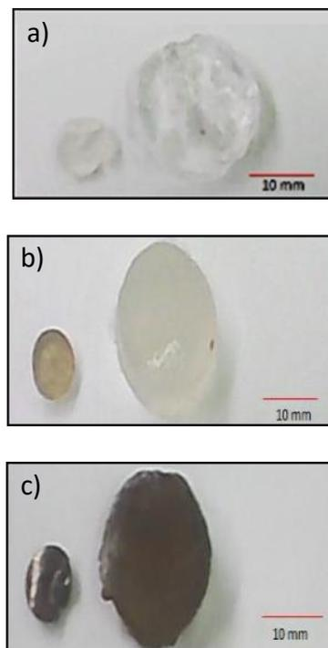
**Fig. 1.** Hydrogels in xerogel condition (left) and fully swollen (right): a) PAAm; b) PAAm/PVA; c) PAAm/PVA/AgNPs
