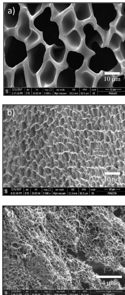
**Fig. 3.** SEM micrographs: a) PAAm; b) PAAm/PVA; c) PAAm/PVA/AgNPs
