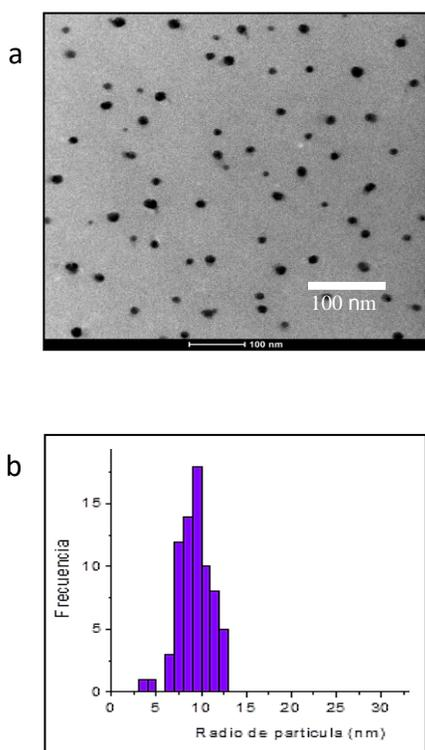
**Fig. 4.** a) TEM micrograph PAAm/PVA/AgNPs, b) AgNPs size distribution
