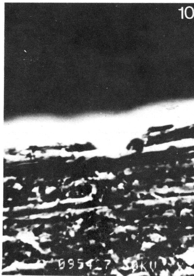
Fig. 10. Scanning electron micrograph showing a cross sectional view of a corrosion pit formed on the alloy surface. As-recived condition. Solution of Cl - , CO 3 -2 , pH=8.
